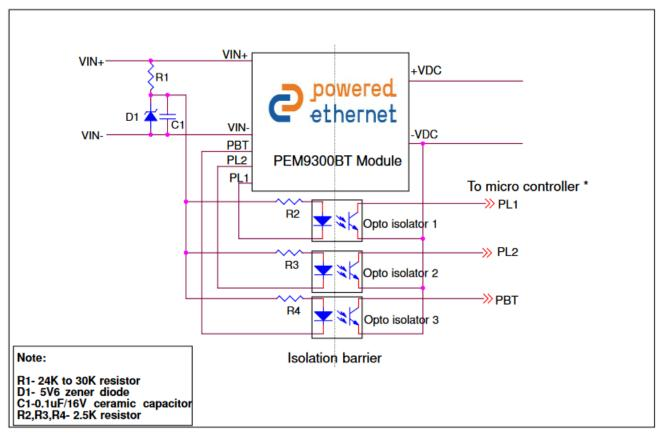
Figure 4- Power level indication connections to host-board
