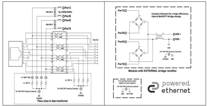
**Figure 1- Typical Input Connections**
