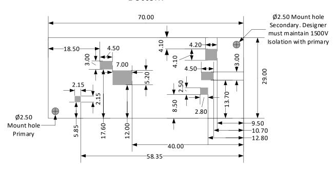
Figure 10- Thermal pad diagram
