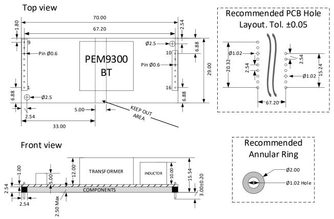
**Figure 11- Mechanical Dimensions**
