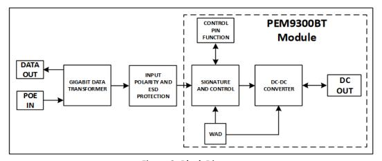
Figure 3- Block Diagram
